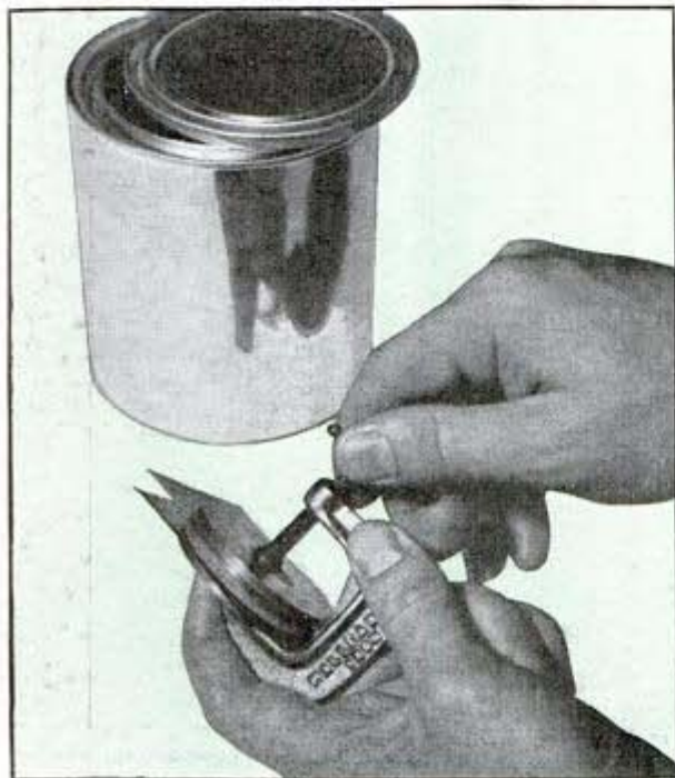
Device for "looking" into steel. Disk to be photographed is clamped between film and brass plates
